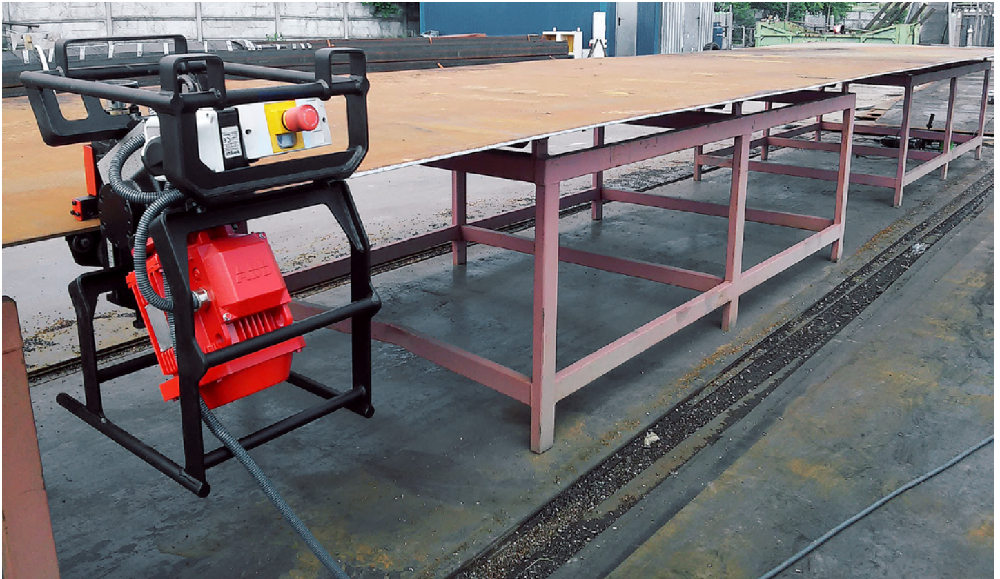
ABM-14 runs along a plate automatically
