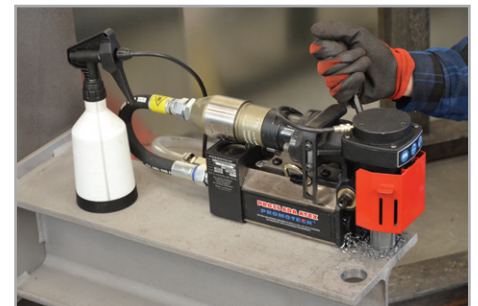
Through spindle cooling system
