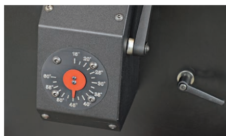
Precise bevel angle adjustment
