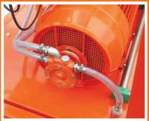
Built in mechanical feed pump.
