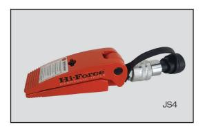
The JS4 hydraulic spreader is the ideal solution for spreading, wedging and prising operations in a wide variety of industrial applications. The compact, low weight, spring assisted return design enables the tool to fit into a gap of 13mm and offers a maximum spread of 84mm. Manufactured from high strength steel, with a maximum pressure of 700 Bar, the JS4 is supplied fitted with a quick connect female half coupler, and can be used with HP110 manual hand pump and HC hose.
