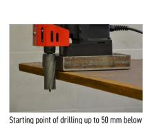
level of a drill base with 100 mm long cutter
