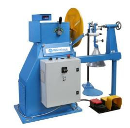
Tooling adjustable for straight and skewed slots. The machine is fitted with a 500mm diameter faceplate and end support with revolving centre which allows it to be used for winding transformers and stator coils. Inclusive of one type TI wire tensioner and dereeler.
